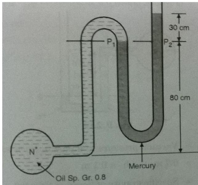
Q14. A simple U-tube manometer containing Hg is connected to a pipe in which a fluid of specific gravity 0.8 and **having vacuum pressure** is flowing the other end of the manometer which is open to the atmosphere. Find the vacuum pressure in pipe, if the difference in Hg level in the two limbs is 40 cm and the height of fluid in the left from the center of pipe is 15 cm below. . (Ans:  $P = -54543.6 \text{ N/m}^2$ )
