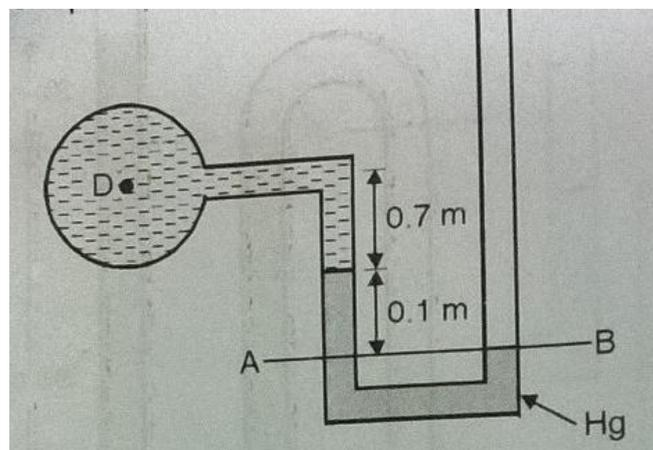
Q16. U-tube differential manometer containing Hg is used to measure the difference in pressure for two pipes C and D as shown in the figure. Pipe C contains carbon tetrachloride of specific gravity 0.8. Pipe D contains oil of specific gravity 0.9. Find the difference of pressure in two pipes. (Ans:  $P_C - P_D = 72.69 \text{ kN/m}^2$ )
