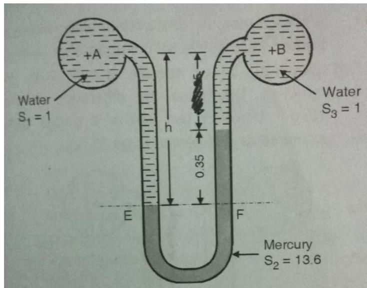
Q18. A differential manometer is connected at two points A and B of two different pipes as shown in figure. The pipe A contains a liquid of specific gravity 1.5 while pipe B contains a liquid of specific gravity of 0.9. The pressure at A and B are  $1 \text{ Kg/cm}^2$  and  $1.8 \text{ Kg/cm}^2$  respectively. Find the difference in mercury level. . (Ans:  $h = 0.18 \text{ m}$ )
