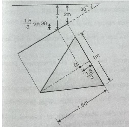
Q10. The tank shown contains water under pressure. Calculate total pressure on side and bottom of tank. Take tank is 2.5 m wide and perpendicular to the plane of paper. ( $F = 882.9 \text{ kN}$ )
