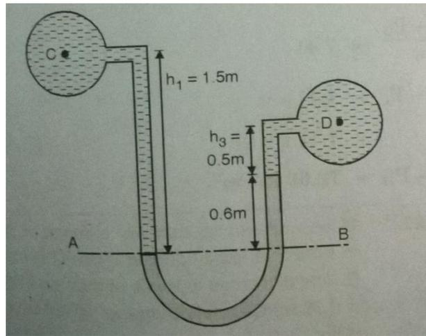
Q17. U-tube differential mercury manometer is connected to horizontal pipe carrying water at two points A and B. the difference in mercury level in the two limbs is 0.35 m. calculate the pressure difference at A and B in KPa. (Ans:  $P_A - P_B = 43.26 \text{ kN/m}^2$ )
